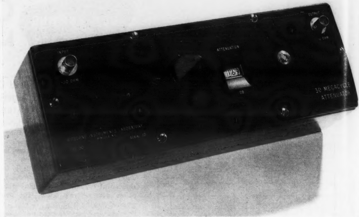
Fig. 1. Attenuation in decibels is read directly at the window in the Type 30 Precision Attenuator.
